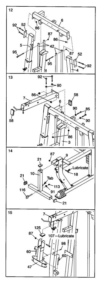
Press a 1 1/2" x 2" Inner Cap (21) into the Right Butterfly Arm (26). Wet the lower end of the Arm with soapy water. Slide a Long Pad (54) onto the Arm.
